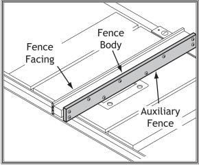
**Figure 60.** Example illustration of an auxiliary fence installed.
